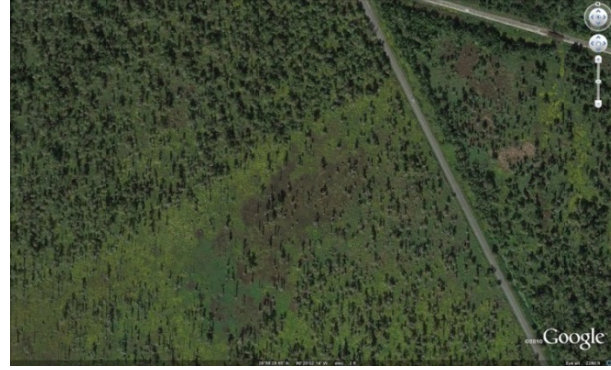
Figure 24 Lineation of the St. Rose Fault expressed as a tree line in the hardwood swamps near the I-310/Airline Hwy intersection west of New Orleans. Google Earth Imagery
