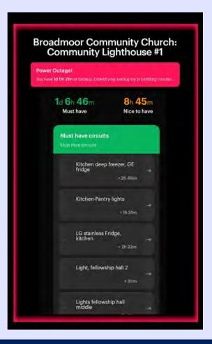
When an outage strikes, the load management system is pre-set to drop unnecessary loads and shift to "must-have" circuits to conserve power.
