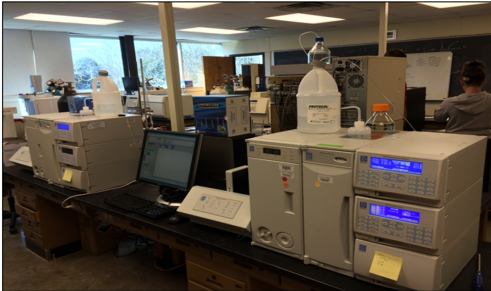
Figure 5: a) Ion chromatographs equipped with electrochemical detector for analysis of minerals and nutrients (anions – left, cations – right) c) Sample chromatogram – cations.
