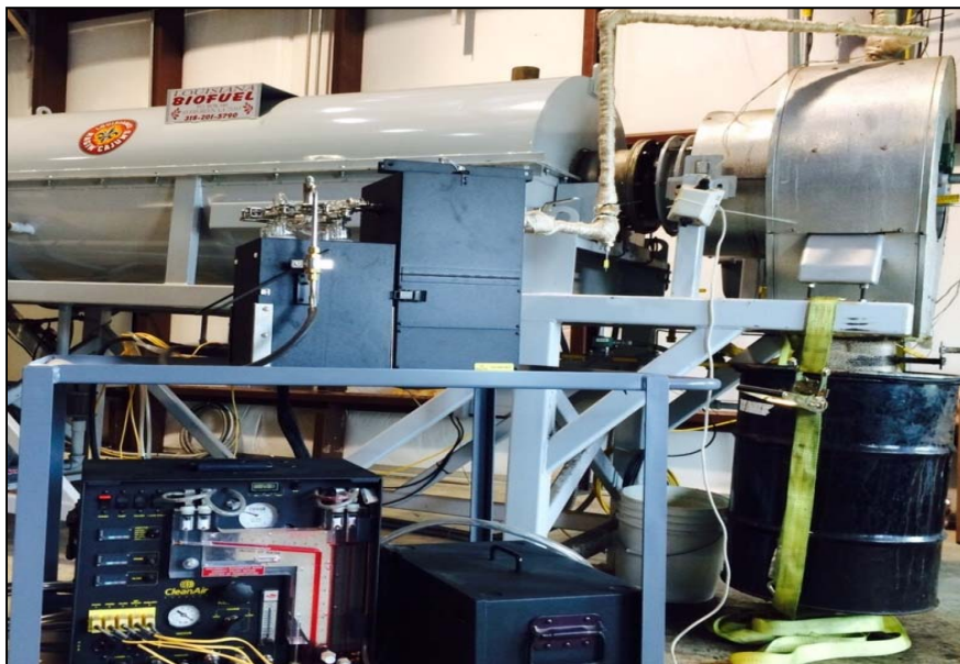
Figure 3: EPA Method 5 sampling system set-up to analyze condensable volatiles and gases
