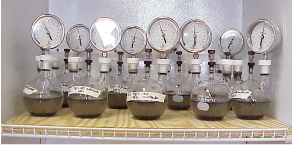
Figure 1: Photograph of Bench-Scale Microcosms.
