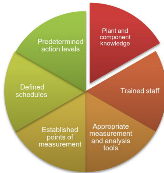
Figure 4-5 Fundamental elements of a condition-based maintenance strategy
