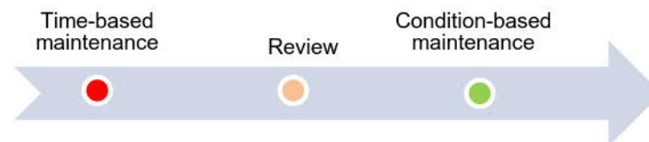
Figure 3-1 Moving from time-based to condition-based maintenance
